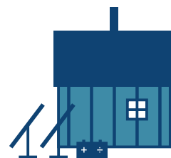
EQALUGAARSUIT Seqernup qinggorneranik katersiviit Panelit 180/67,5 kWp Batteriillu 167 kWh/100 kVA
